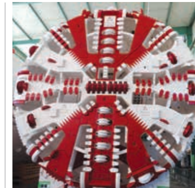
Tunnel-boring machine (TBM)
